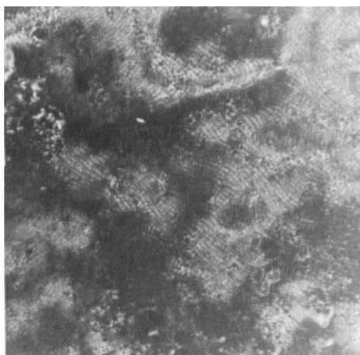
FIGURE 2 Smectic C Schlieren texture with two superimposed Sm C layer undulation instabilities (cross-hatched patterns 4 ) in a thin (26 microns) NOBA film produced by first and second-order effect after rapid cooling of the twisted nematic phase. These Sm C patterns usually appear in the lower temperature range of the Sm C phase. Cross nicols, each side of the photo corresponds to 510 microns.
